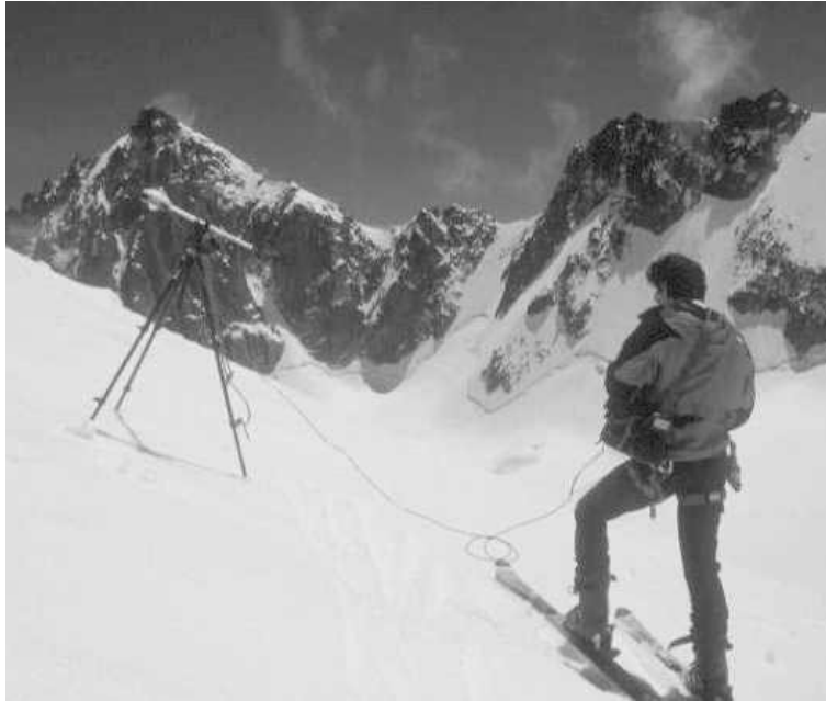
Figure 12: Albedometer setting. The white oval, above and left the camera tripod is the albedometer, made up of two Kipp & Zonen opposed pyranometers. The output is read in two voltmeters connected at the extreme of the cable, hold by the skier-operator in the image.
