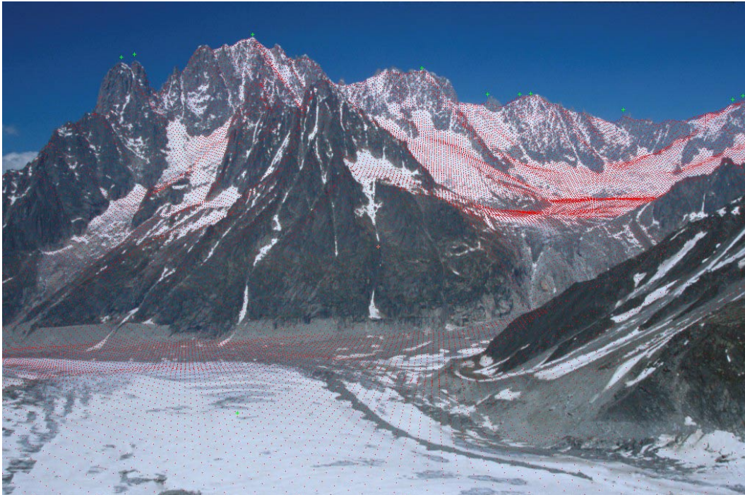
Figure 5: Super imposition of the perspective projection of a DEM of the Mer de Glace glacier (figure 4) over a photograph of the area. Red dots are the perspective projections of the original DEM grid cells, green dots are ground control points. The photograph is taken from the Refuge du Requin looking east-northeast.
